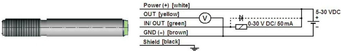
Connection analog with open collector alarm output
